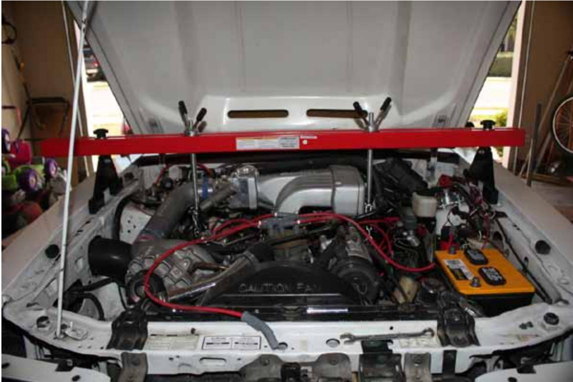
4. Use an engine support beam or a piece of wood on a floor jack to raise the engine high enough to get the motor mount stud out of the k-member.
