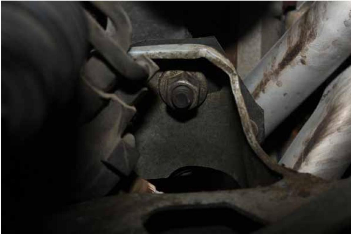
3. Remove nuts (1 each side) from the bottom of the motor mounts.
