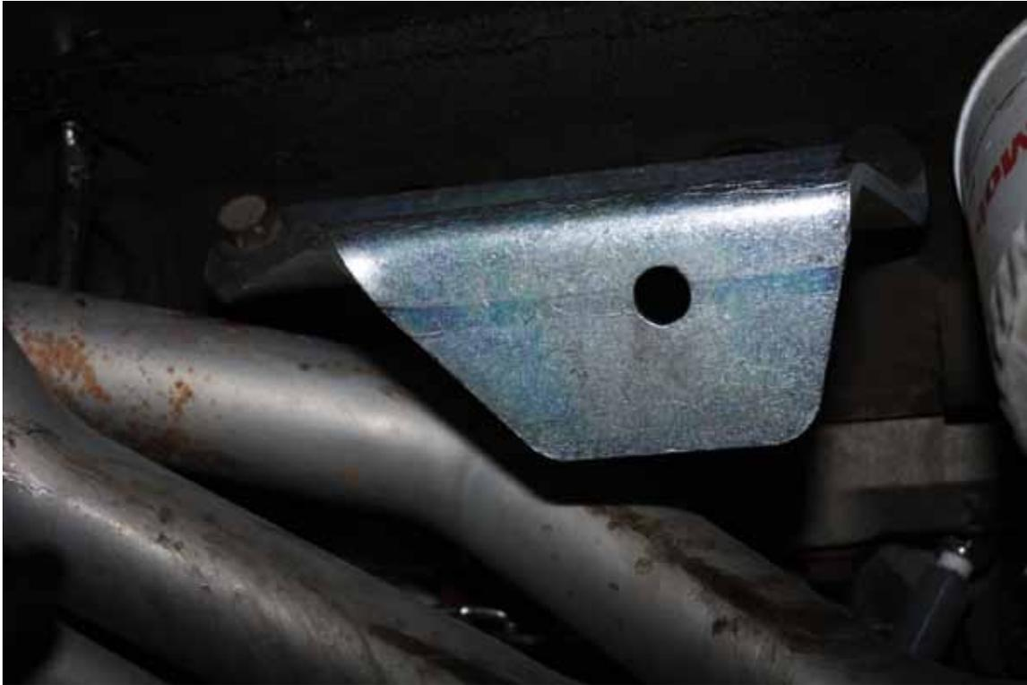
6. Bolt the solid mounts to the engine block.
