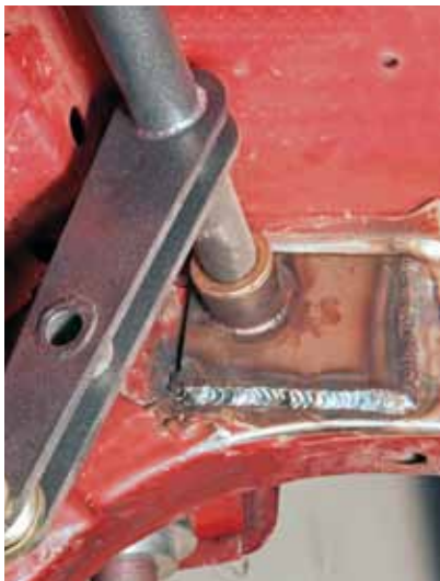
The antiroll bar features oil light, self-lubricating bronze bushings and comes in regular, X-treme, and tailpipe-clearing configurations.
